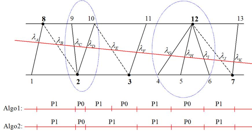
**Figure 6.** Example of edges cut by an interface. Dotted edges are non-vital. Groups of connected vital edges are circled. The final multiplier approximation (P0 or P1) is plotted on the interface for both algorithms.
