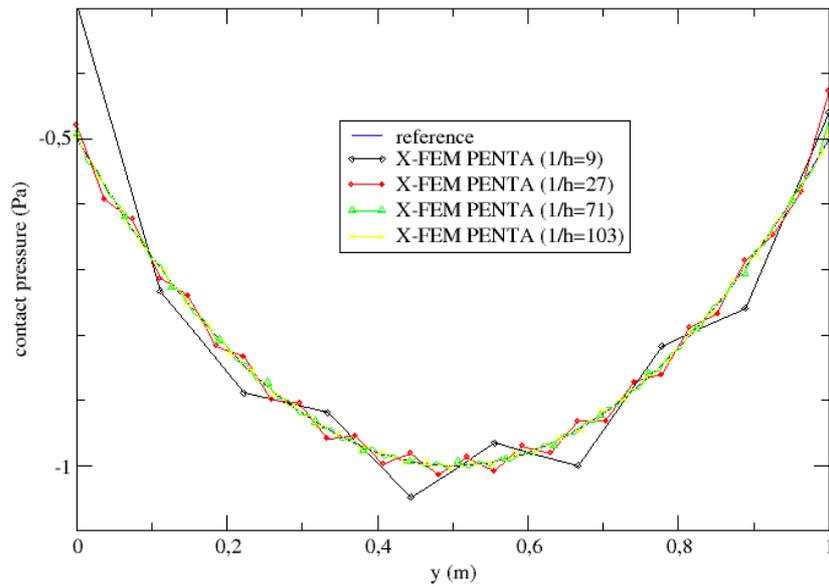
**Figure 7.** Reduction of the contact pressure oscillations as the mesh gets finer.
