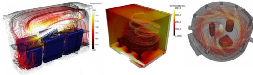
*Figure 1. Streamlines and isotherms inside industrial furnaces*
